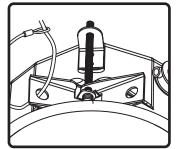
6. If required, attach seismic restraint system to the sheet-metal tab on the rear panel of the speaker, then to reinforced structure (safety cable not included).
